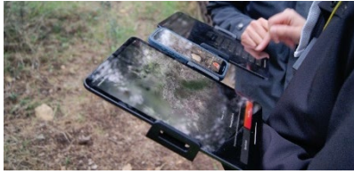
Figure 2. Photogrammetric acquisition base integrating the GS-iPad on the left, SfM-iPhone in the center, and LiDAR-iPad on the right.
